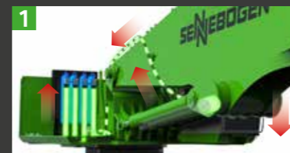
1 Boom lowers, gas compresses
